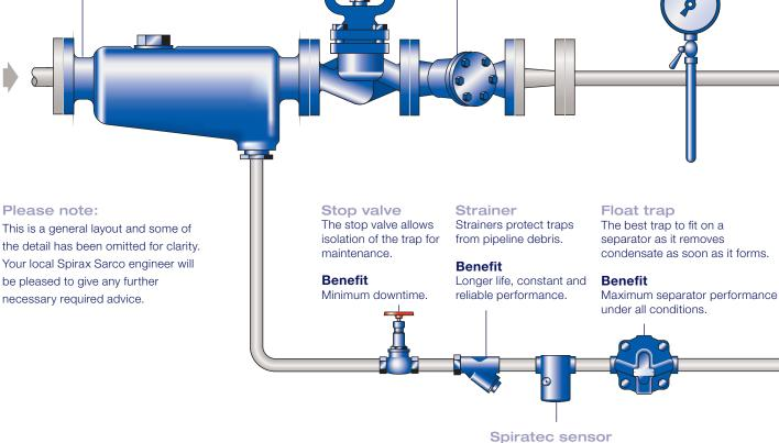
This enables continuous monitoring of the trap performance.
